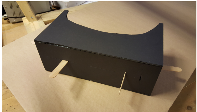
Figure 21: Second version body console with side panel controllers.
