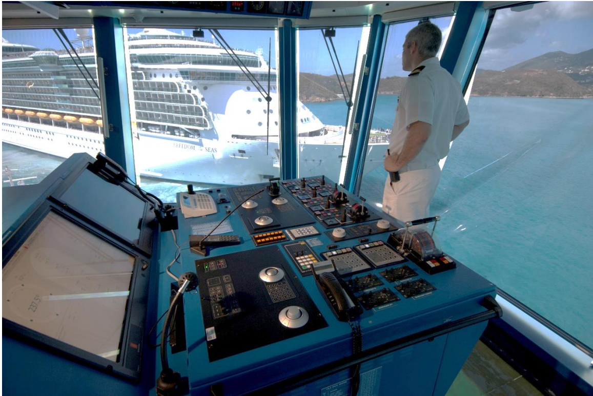
Figure 3-1: Traditional ship bridge wing. Courtesy of Kongsberg Maritime. Retrieved from https://www.km.kongsberg.com , 23.05.2016
