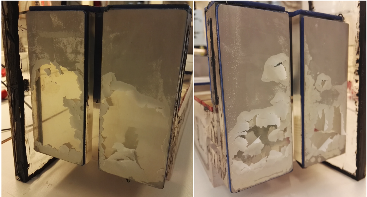
Figure 5.12: Surface picture of samples 1, 2 and parts of sample 13. The surface has not been touched prior to these pictures. This layer is assumed to be a calcareous deposit.
