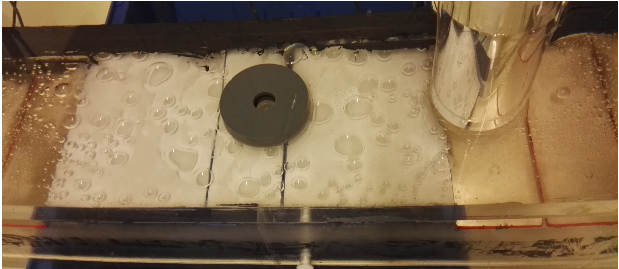
Figure 5.10: Pictures of metal samples inside the test cell at the end of exposure to the seawater electrolyte.
