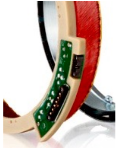
Figure 35 - Typical Circuitboard Connection for ThinGap™ Stators - https://www.thingap.com/standard-products/
