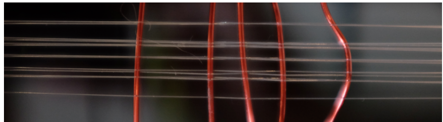
Figure 18 - Bent Wires in Grid
