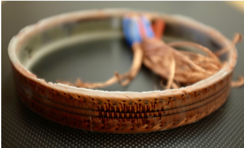
Figure 63 - Two Layer Vacuum Infused Stator
