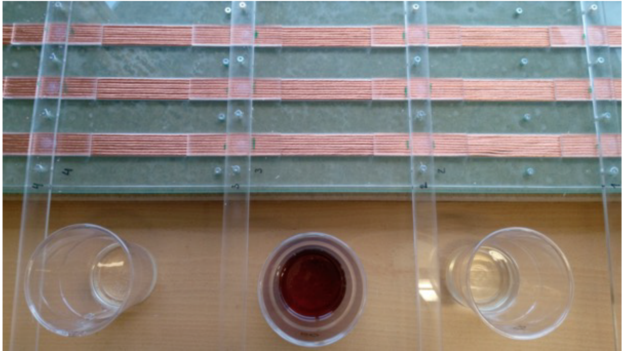
Figure 21 - Laser Cut Molds with Pooling of Active Area
