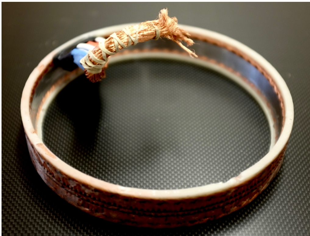
Figure 64 - Three Layer Vacuum Infused Stator
