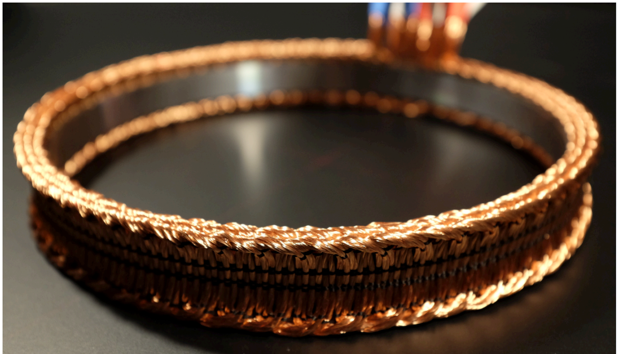
Figure 56 - Three Layer Rolled-up Stator
