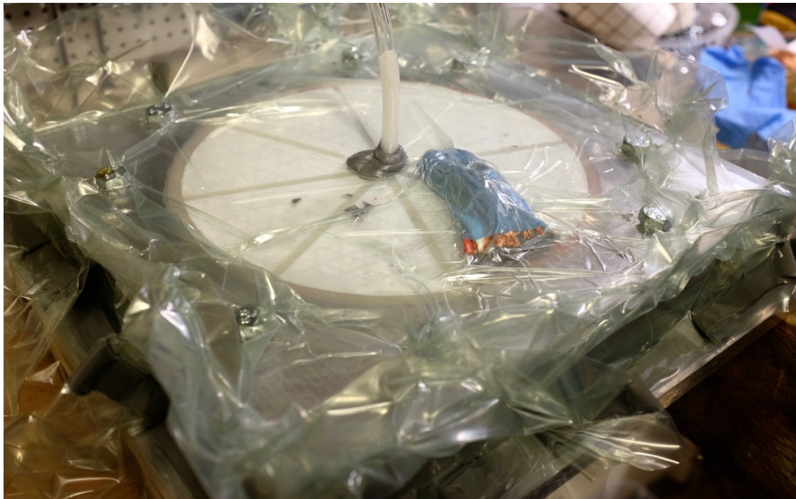
Figure 62 - Vacuum Infusion Prototype with Bagging for Sealing
