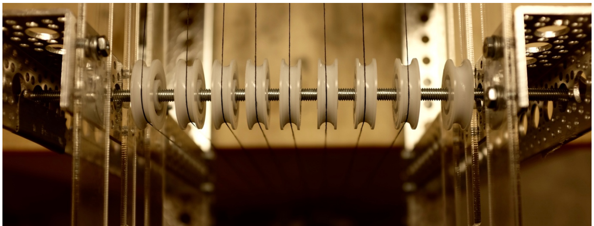
Figure 53 - Warp Yarns with Weight Tension
