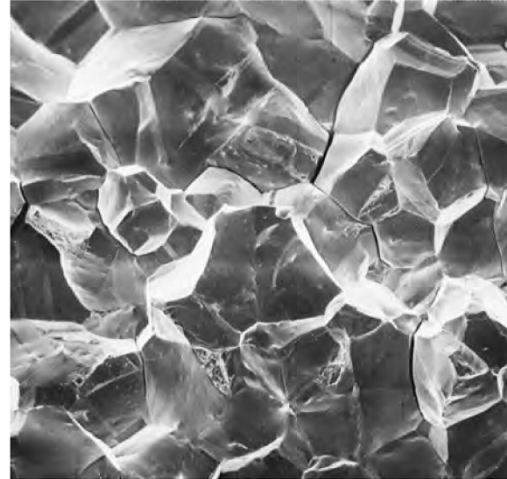
Figure 2.7: SEM of a intergranular fracture surface. Magnification 50X. 24
