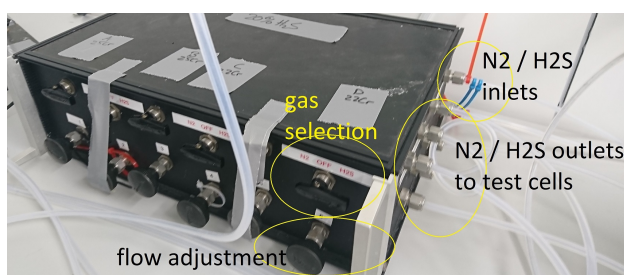
Figure 3.5: Control manifold used to adjust flow and input gas to cells. Yellow circles from upper right to lower left show the input connection points for gas, the output lines to different test cells, gas selection valve ( N_2 , closed or H_2S ) and flow control valve.
