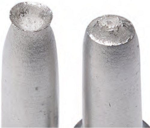
Figure 2.2: Ductile Cup-and-cone fracture of an aluminium specimen. 24
