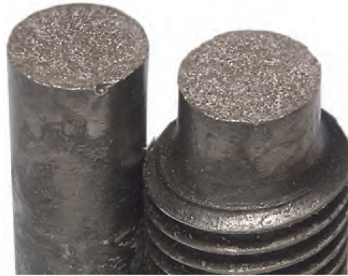
Figure 2.3: Brittle fracture surface of a mild steel. 24
