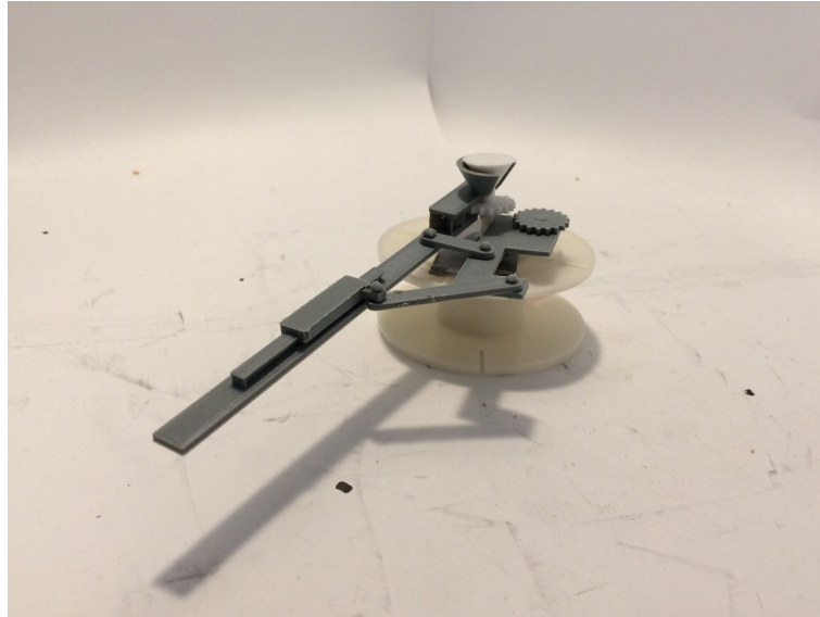
Figure 3.18: Stabilized external gripper 3D-print
