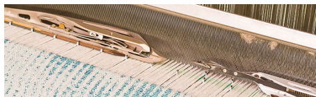
Figure 2.2: The receiving rapier meets the feeding rapier mid-way across the warps
