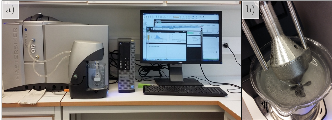
Figure 3.7: a) Malvern Mastersizer 3000 laser diffraction particle size analyser with Hydro EV wet dispersion. b) Close-up on the Hydro EV stirrer (head raised), showing problems with floating graphite (tailings sample).
