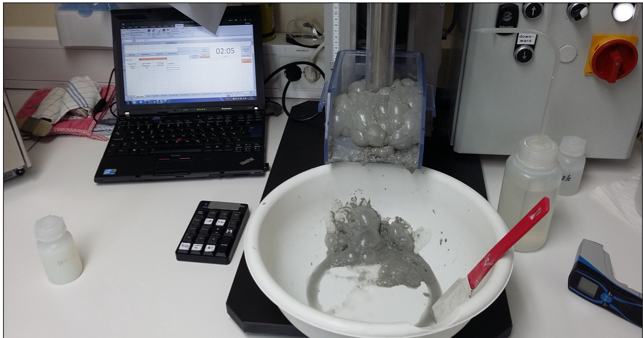
Figure A.1: Flotation Log in use. Wireless remote located below the laptop.
