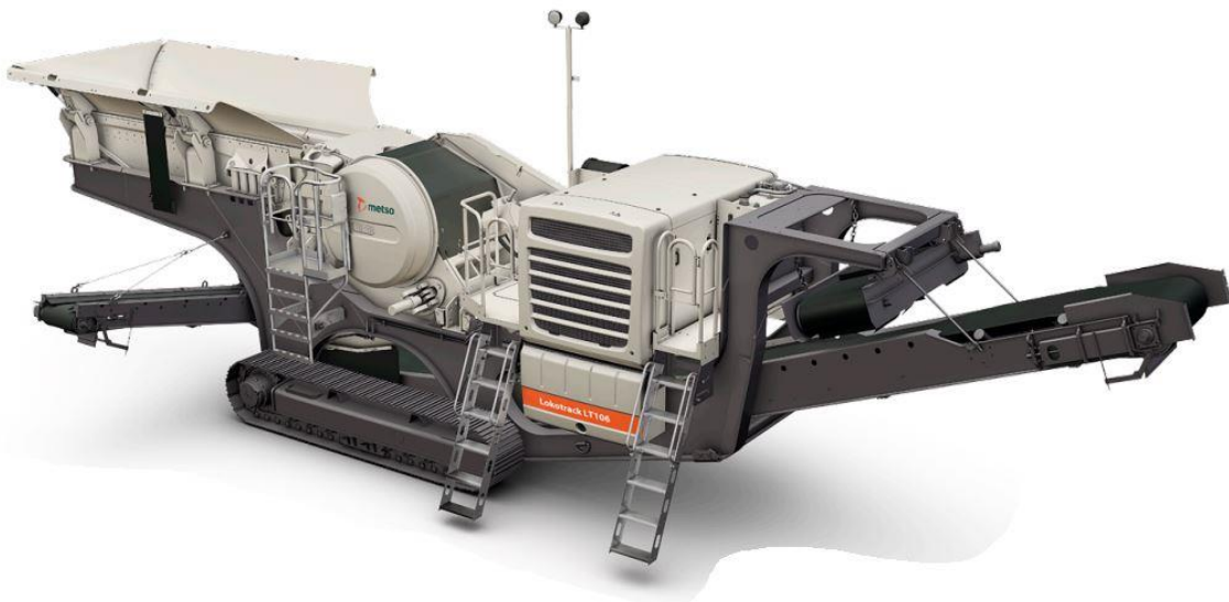
Figur 14: Lokotrack LT106 mobilknuser (Metso, 2016)
