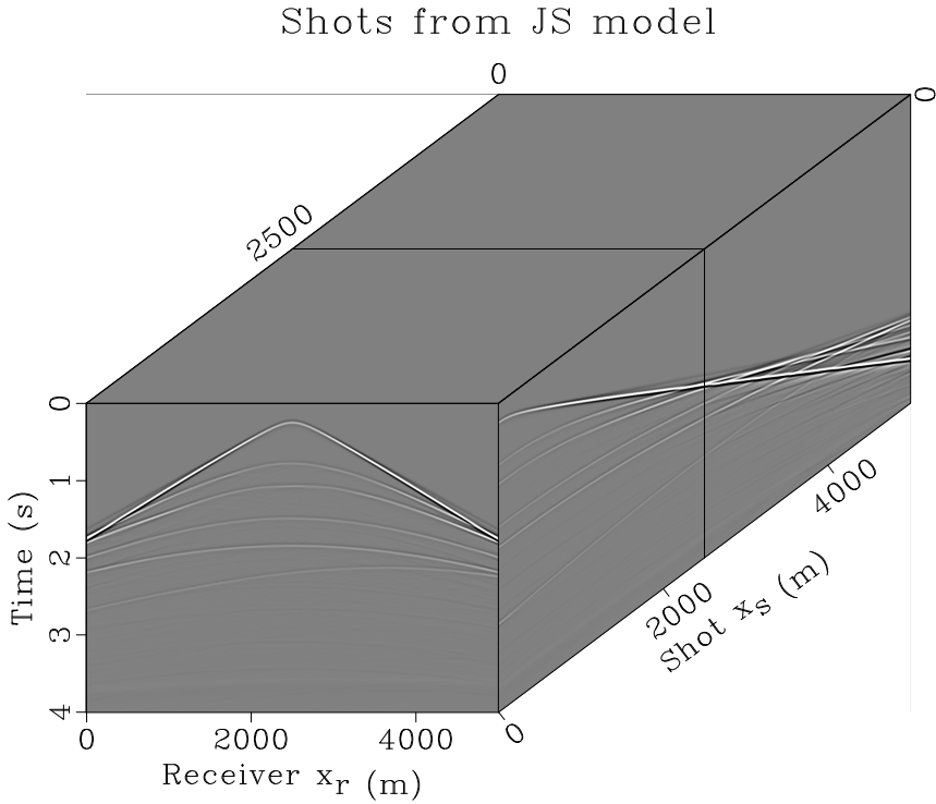
Figure 6.12 Cube of shots modelled using the velocity and density models in figure 6.11
