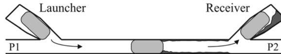
Figure 2.11: Pig driven by pressure difference across it ( P1 > P2 ) (Quarini and Shire, 2006)
