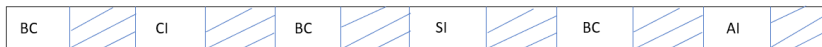
Figure 5.2: An example on how the chemicals can be transported, when biocide is injected every other time
