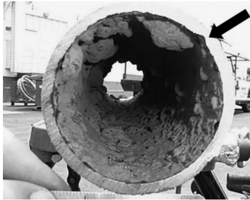
Figure 2.6: Pitting corrosion due to MIC in a carbon steel water pipe (Skovhus et al., 2017)
