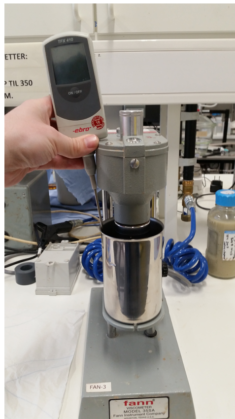
Figure 4.1: Setup for viscosity measurements
