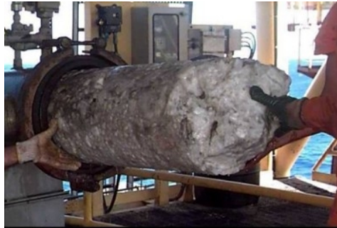
Figure 2.1: A large gas hydrate plug formed in a subsea hydrocarbon pipeline (Heriot-Watt University, 2017)
