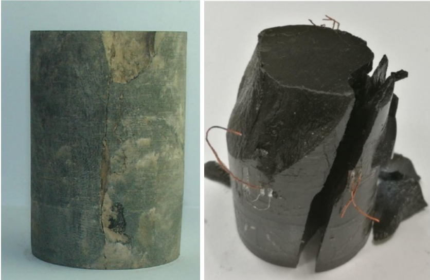
Figure 0.13: Core sample before (left) and after (right) the test. The sample is cracked before being tested.
