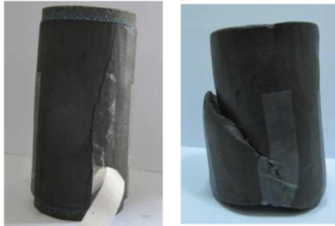
Figure 0.22: The failed samples. TCP1 left and TCP3 right (Yu, et al., 2015).
