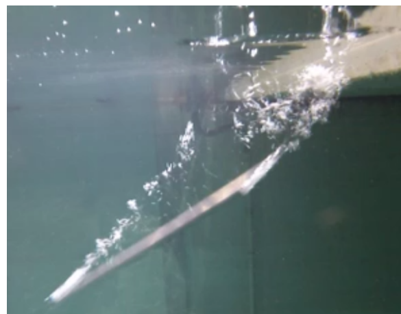
Figure 5.11: Drop angle: 45^\circ . Cavitation bubbles on the upper front and the back end of a type 3, dropped with COG 63 cm above the water surface with a drop angle of 45^\circ . Figure 5.12: Drop angle 60^\circ . Cavitation bubbles on the upper front and the back end of a type 3 cylinder, dropped with COG 63 cm above the water surface with a drop angle of 60^\circ .
