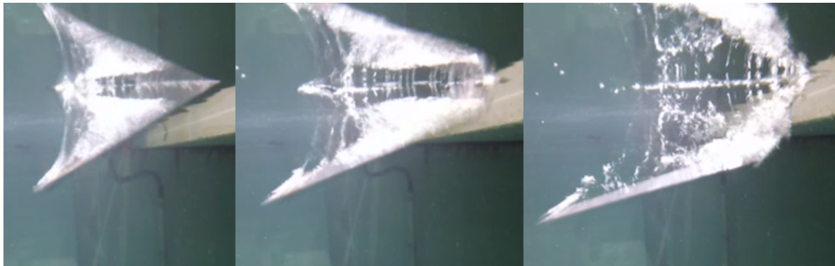
Figure 5.10: Water entry of a cylinder of type 3 dropped with COG 63 cm above the surface with a drop angle of 45^\circ . The upper part of the picture is the mirrored reflection from the free surface.
