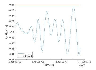
Figure 3.8: Comparison of z position and desired z position at intermediate velocity
