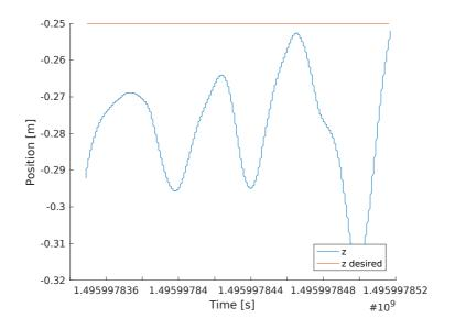
Figure 3.12: Comparison of z position and desired z position at high velocity
