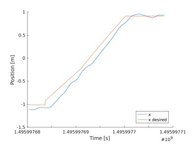
Figure 3.6: Comparison of x position and desired x position at intermediate velocity
