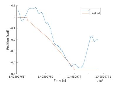
Figure 3.9: Comparison of heading and desired heading at intermediate velocity
