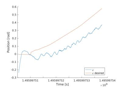
Figure 3.5: Comparison of heading and desired heading at low velocity
