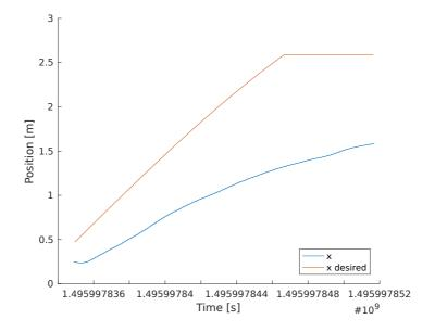
Figure 3.10: Comparison of x position and desired x position at high velocity
