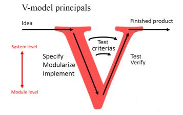
Figure 1.1: Illustration of the V-model software development method (Øyvind Stavdahl, 2016)
