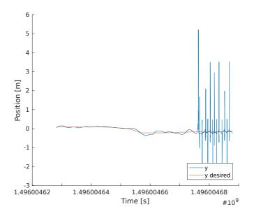
Figure 4.4: Comparison of y position and desired y position
