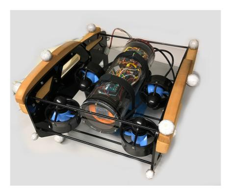
Figure 2.7: The uDrone ROV with Qualisys passive reflectors
