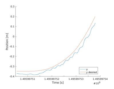
Figure 3.3: Comparison of y position and desired y position at low velocity
