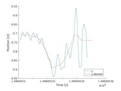
Figure 4.12: Comparison of y position and desired y position
