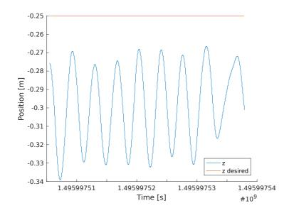
Figure 3.4: Comparison of z position and desired z position at low velocity
