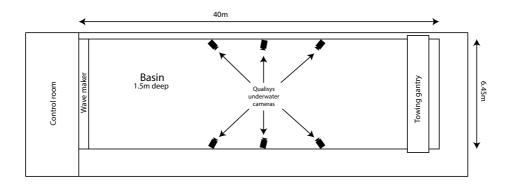
Figure 2.1: Drawing of the Marine Cybernetics laboratory
