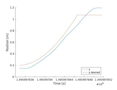
Figure 3.11: Comparison of y position and desired y position at high velocity
