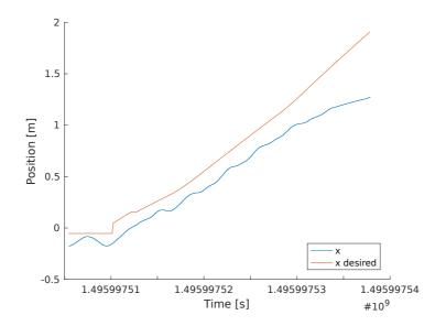
Figure 3.2: Comparison of x position and desired x position at low velocity
