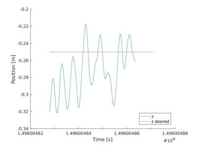
Figure 4.9: Comparison of z position and desired z position
