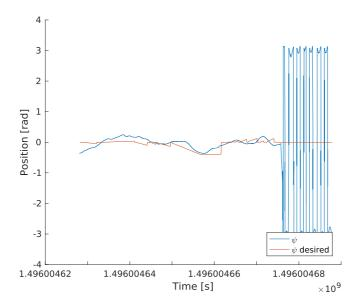
Figure 4.6: Comparison of heading and desired heading
