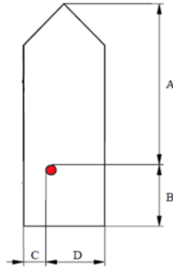
Figure 4.2: Location of antenna given by parameters A, B, C and D in AIS messages
