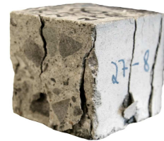
Figure 4.21: Cube 27-8 after testing.
