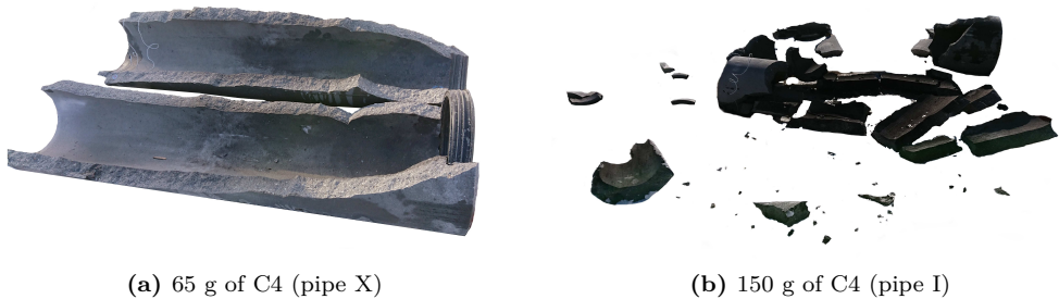
Figure 6.28: Damage of two of the larger plain concrete pipes.
