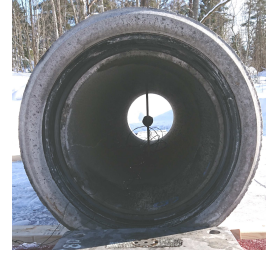
Figure 6.8: Spherical charge placed centrally within pipe.
