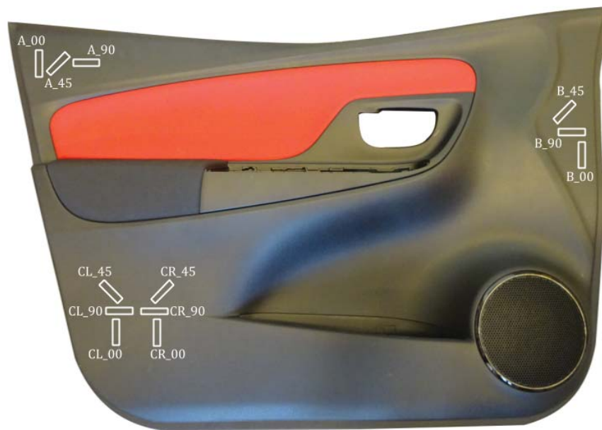
Figure 3.16: Representative tensile specimen outline from which the door trim cutouts were extracted
