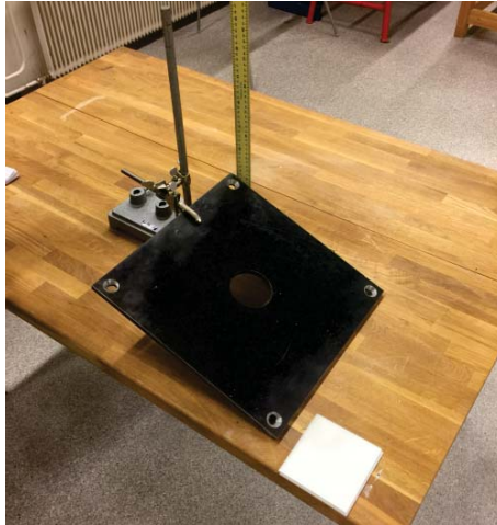
Figure G.0.2: Inclined plane test setup
