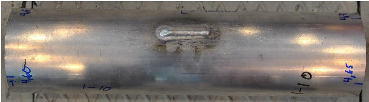
Figure 7.3 – Weld on surface for alloy 6082-T6, D=100 mm, t=4.8 mm. L_w = D/2 .
