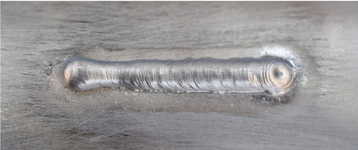
Figure 6.6 – A weld on alloy 6060-T6, D=100 mm, t=4.8 mm. The length of the weld is D/2.
