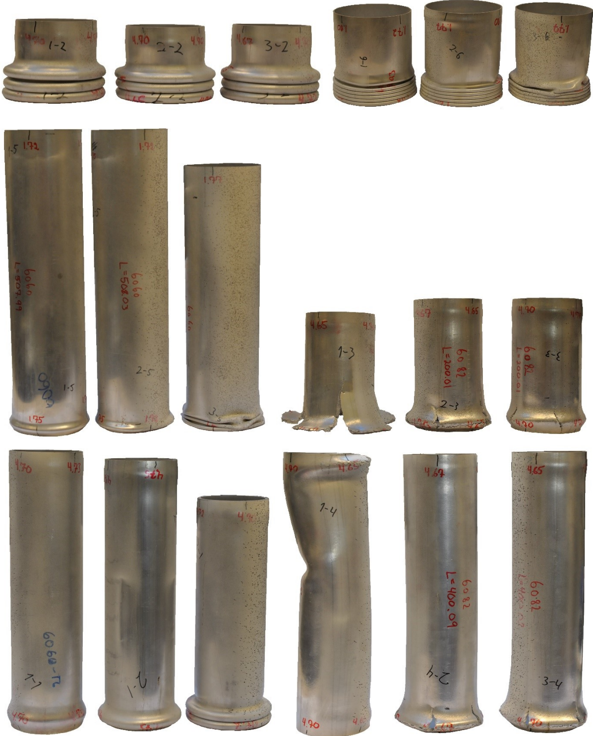
Figure 7.2 – Results from compression tests of unwelded cross sections.
