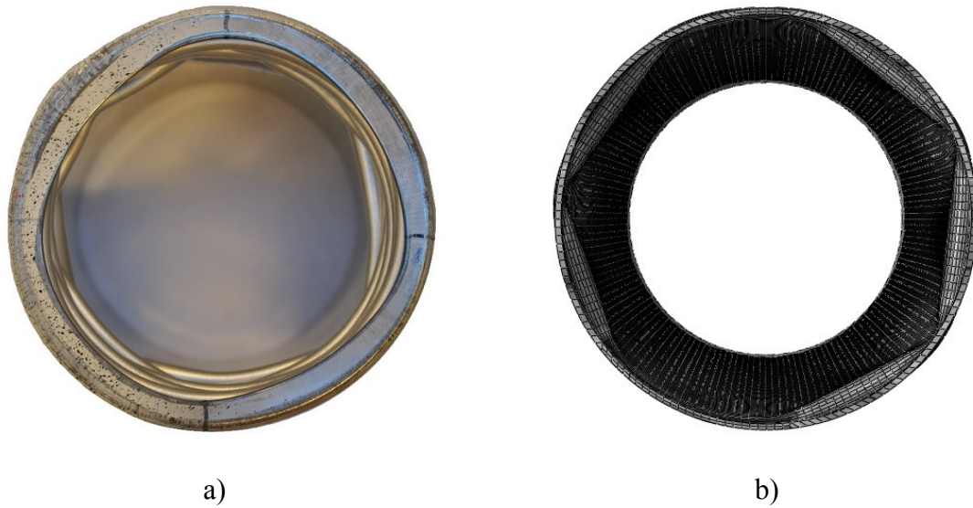
Figure 9.26 – Non-symmetrical/diamond form of a) laboratory results and b) numerical results of unwelded alloy 6060-T6, D=127 mm, t=1.8 mm and L=508 mm.
