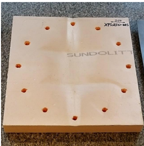
a) With a front plate (XPS-250-07S)
