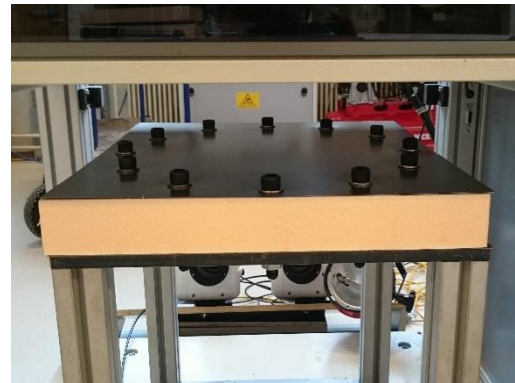
c) Sandwich test specimen bolted in place
