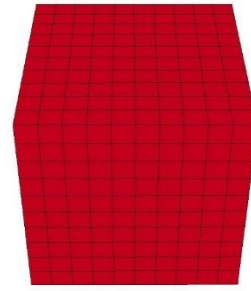
b) Foam test specimen meshed in LS DYNA
