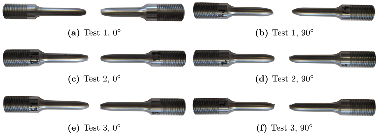
Figure 3.9: NVE 36 specimens post fracture.
