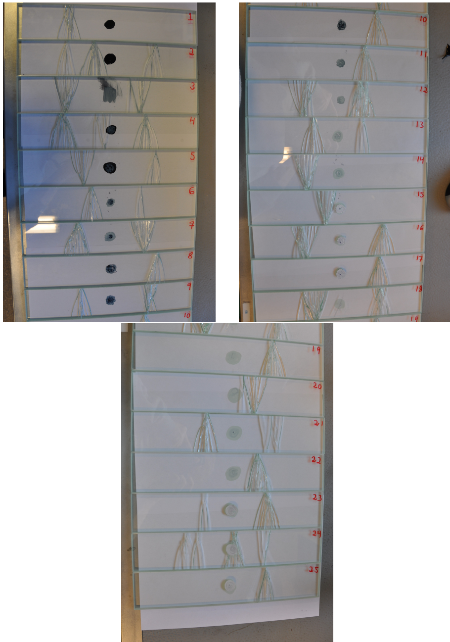
Figure A.3: Large four point bending test samples (300 × 60mm)
