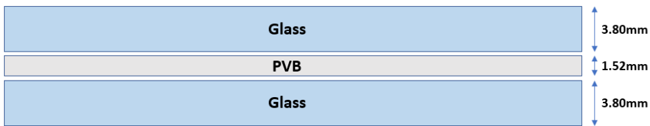
Figure 4.10: Cross section of the laminated glass panes tested
