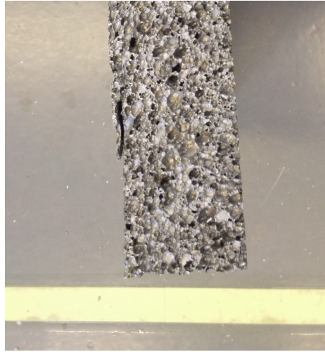
Figure 6.11: Flaw in test specimen 2A
