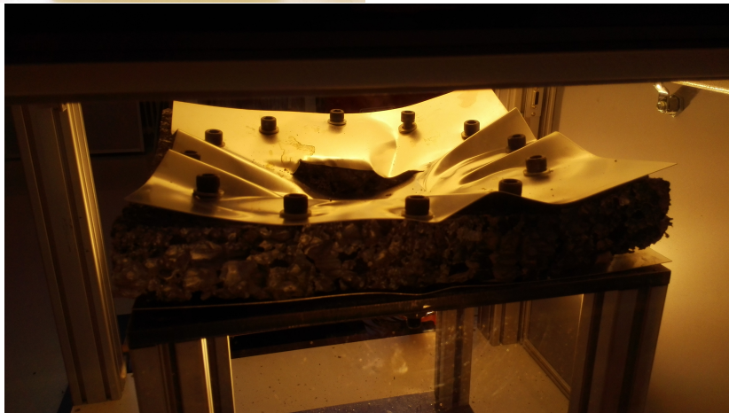
Figure 6.12: Test set up for the drop tower experiments
