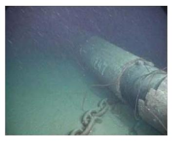
Figure 1.1: A pipeline impacted by an anchor [4].
