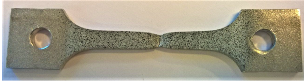
Figure 3.16: Deformed geometry of a representative test from the flat specimen L20. The speckle pattern spray-painted on to the gauge region prior to the test is visible.
