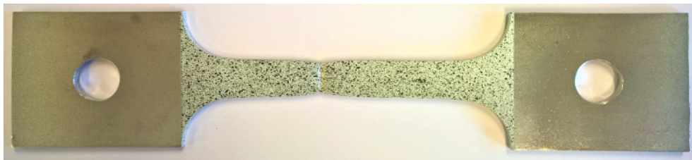
Figure 3.19: Deformed geometry of a representative test of the flat specimen L50. The speckle pattern spray-painted on to the gauge region prior to the test is visible.
