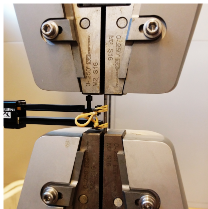
Figure 5.14: Uniaxial tension test of reinforcement mesh.
