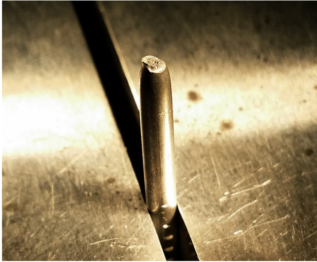
Figure 5.16: Fractured test specimen.
