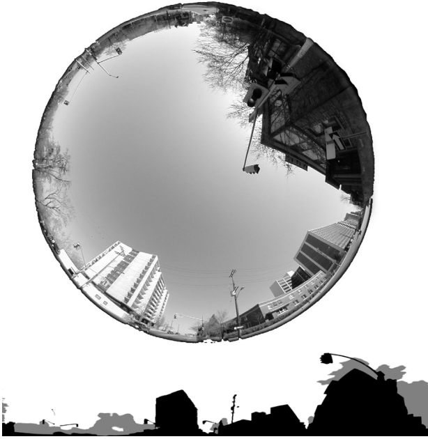
Figure 1. Top: Fisheye picture. Bottom: unwrapped picture sorted into clear (white), shadowed (gray) and blocked (black) states
