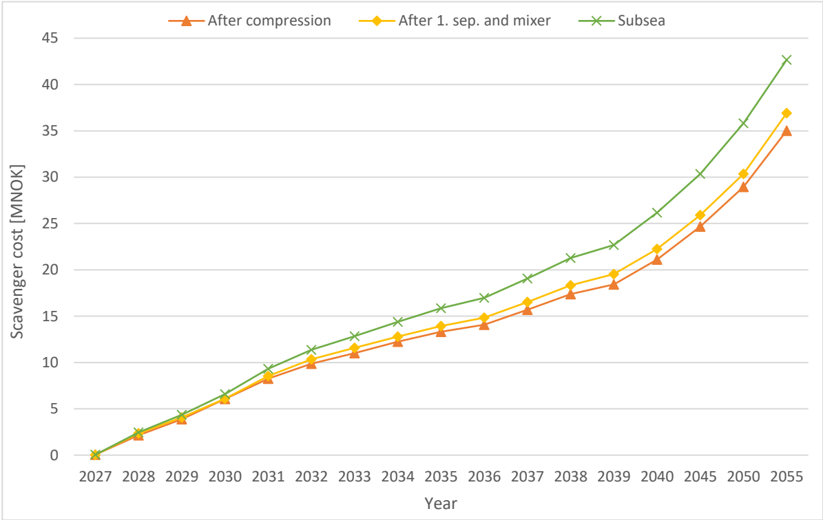
Figure 8-3: Scavenger chemical cost. Phase 2
