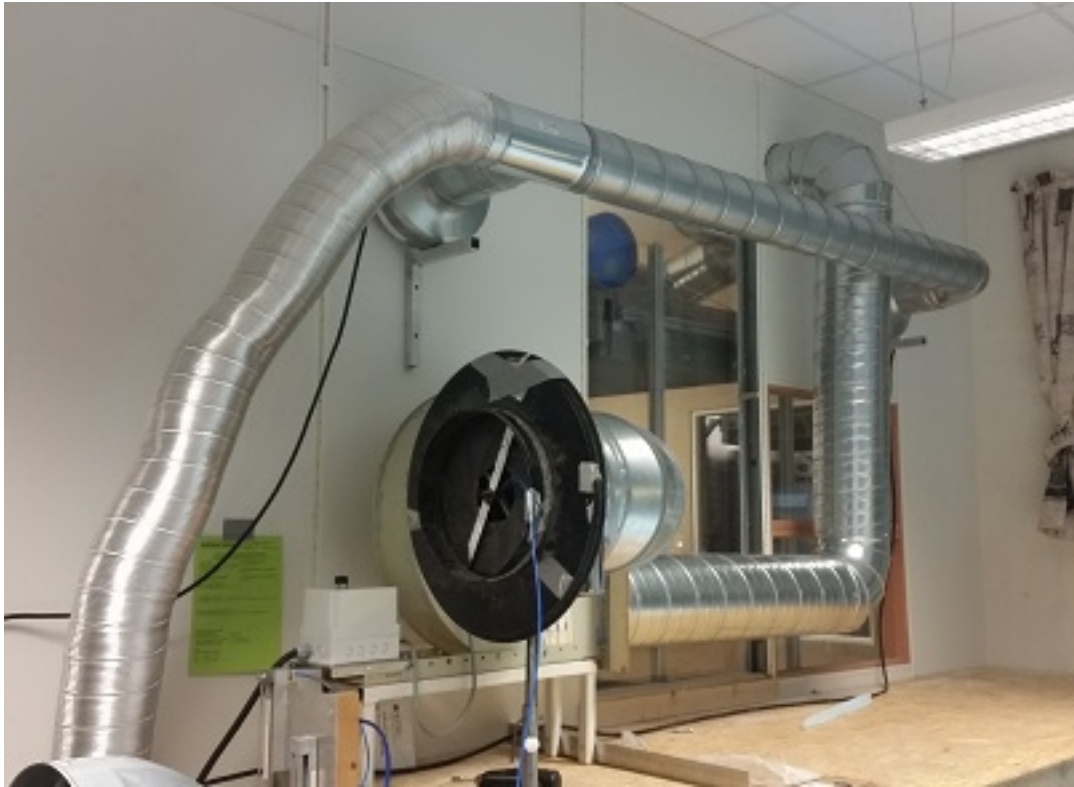
Figure 41: The supply fan for LAF diffuser and exhaust pipe on outside of experimental room
