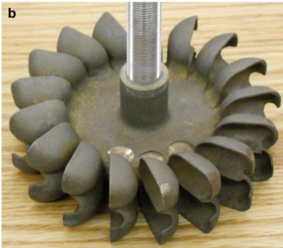
Figure 3.27: Photos of a Turgo turbine (a) and a Pelton turbine (b) [10].
