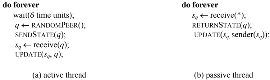
Figure A.2. The gossip paradigm. Notation: q is the remote peer; s_q is the state received from q (from [Mon04]).
