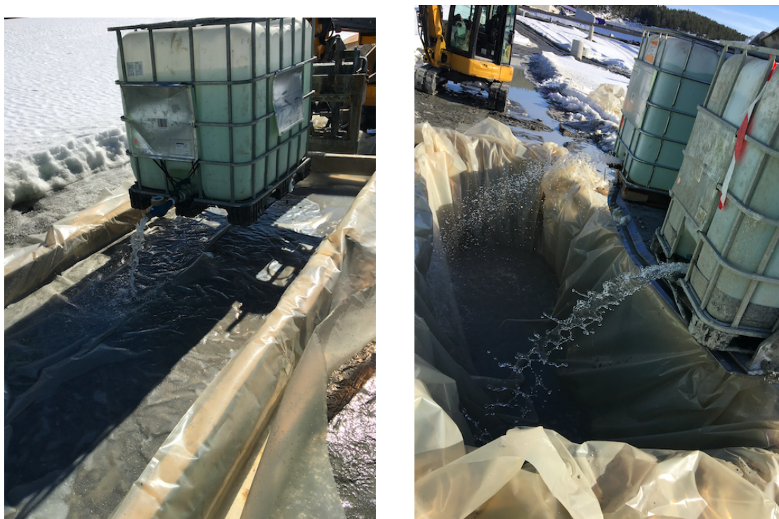
Figure 3.18 – Right: Filling frame with water, volume measured through flowmeter. Left: Pit filled with water measured as sum of several flowmeters
