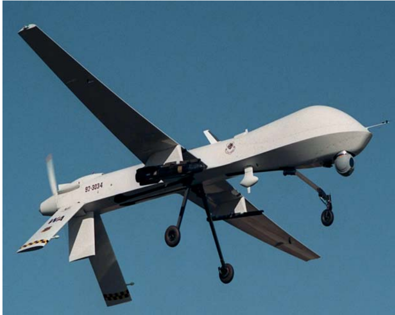
Figure 1.6: An MQ-1 Predator armed with an AGM-114 Hellfire missile flies a training mission (Courtesy to the U.S. Airforce).
