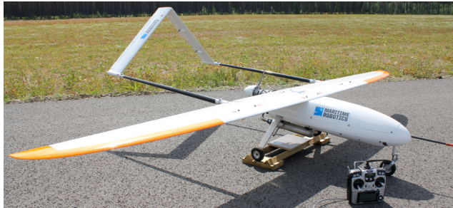
Figure 3.5 Maritime Robotics’ Penguin B from UAV Factory that was used during the experiments.
