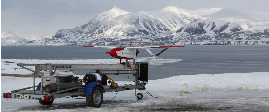
Figure 1.4 A launch system for the CryoWing fixed-wing aircraft operated by Norut (2014) in Longyearbyen, Svalbard, May 2011.
