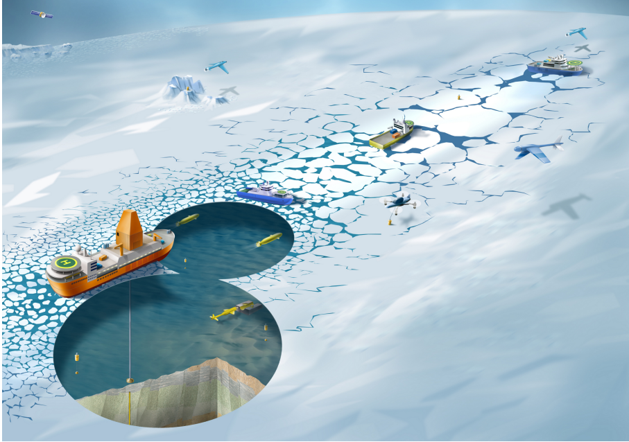
Figure 1.3 Illustration of a possible future Arctic dynamic positioning operation that consists of many important components, including icebreakers, unmanned underwater vehicles, and unmanned aerial vehicles. Picture courtesy of Bjarne Stenberg.
