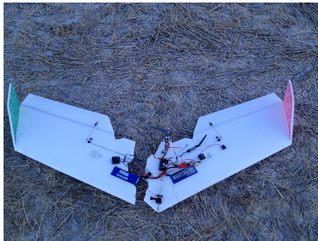
Figure 8.10: UAV After Failed Take-off
