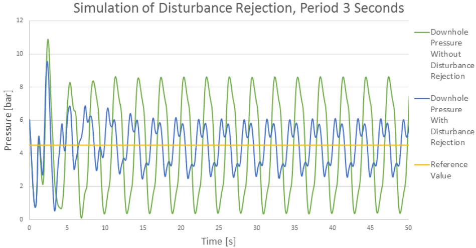
Figure 7.10: The disturbance rejection of waves with a period of 3 seconds, simulator test.
