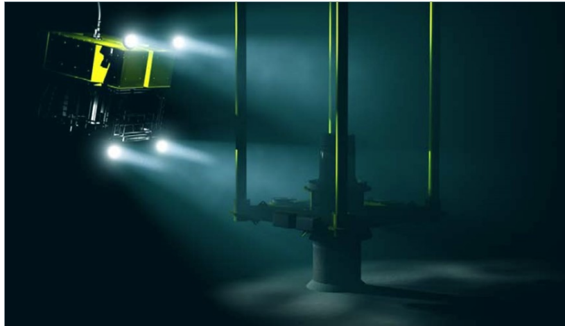
Figure 4: The figure shows a ROV and the wellhead (top of the well), before the XT is installed (Source: Aker Solutions)
