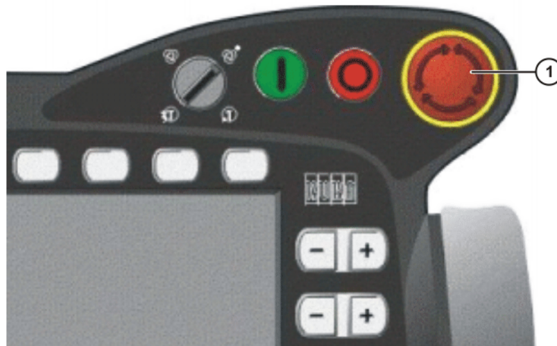
Fig. 5-3: EMERGENCY STOP button on the KCP
