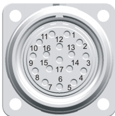
Fig. 9-10: M23 connector, 17-pole, view from contact side
