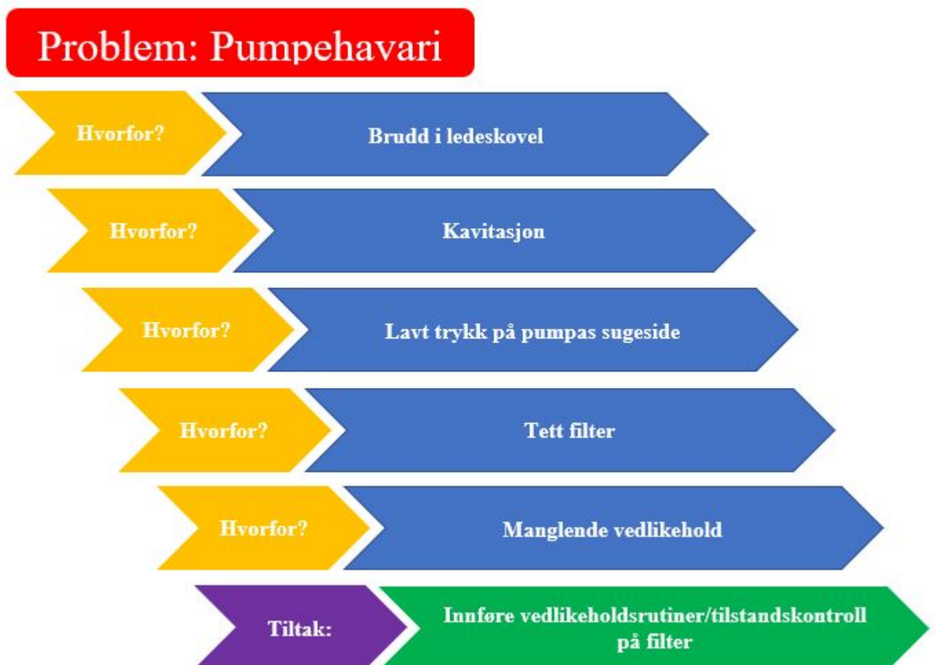
Figur 12: 5-why for pumpehavari (Bye 2009)
