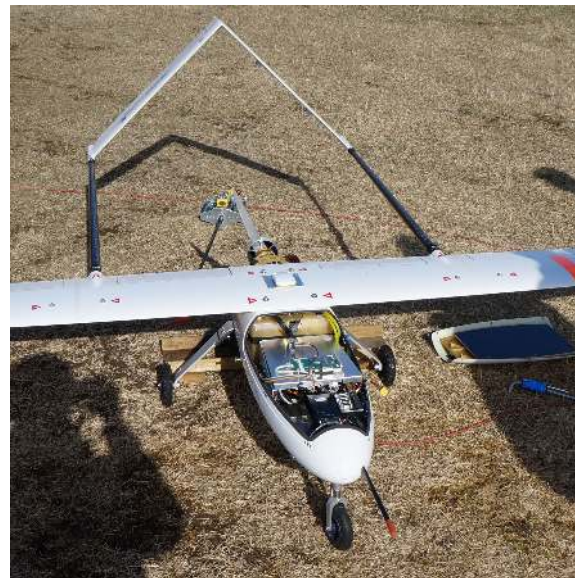
(d) Installation of the payload in the UAV finished.
