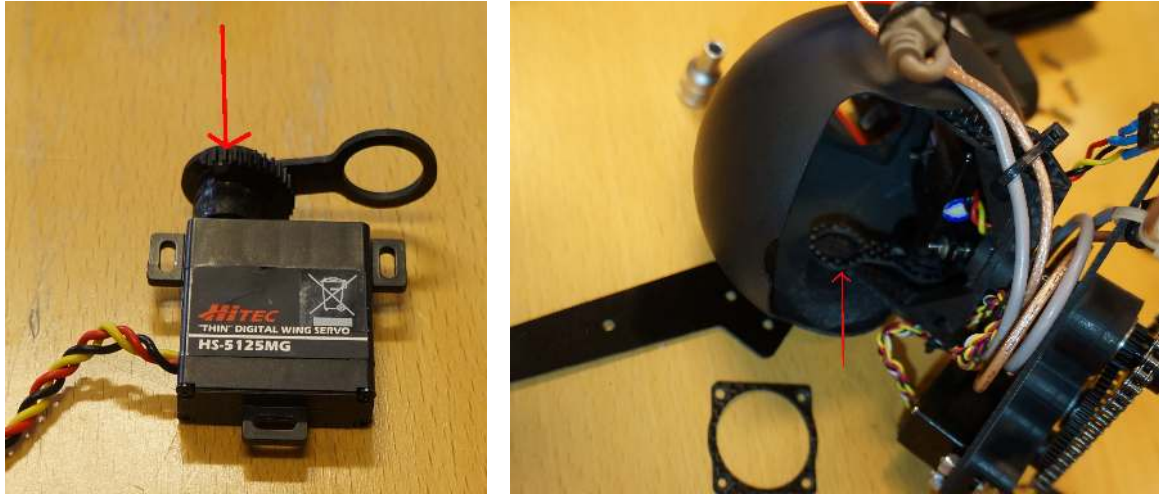
Figure B.15: Replacing tilt servo in the gimbal.
