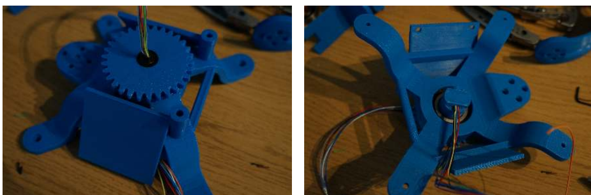
Figure B.18: Installing the slip ring in the geared yaw shaft.
