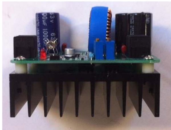
Figure 9.7: The new overpowered step-up converter with large heat sink.
