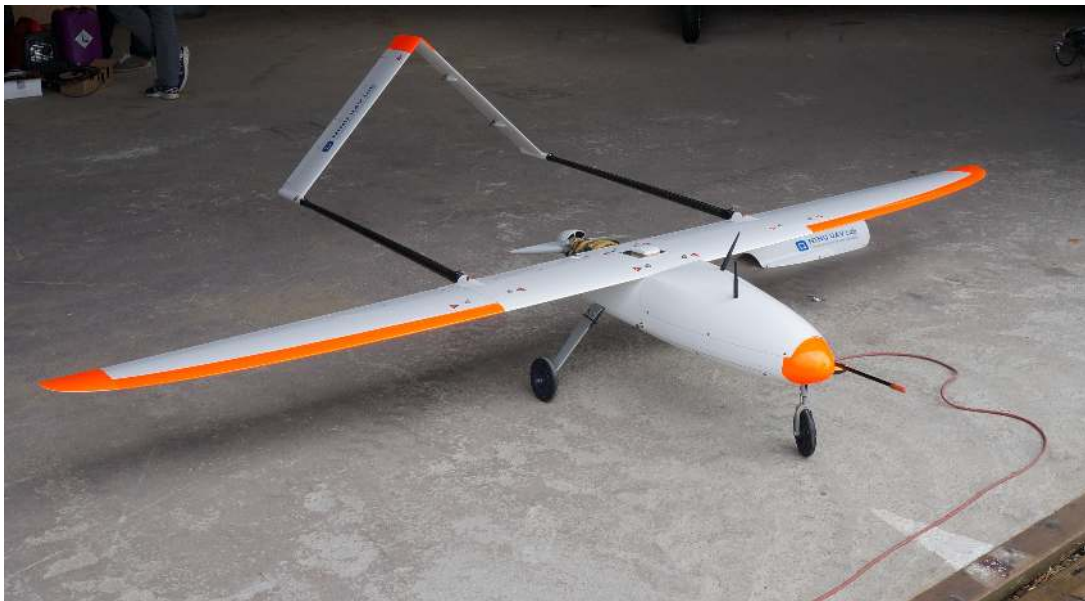
(b) Penguin B with payload installed.
