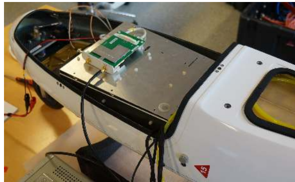
(b) Payload housing mounted in the UAV, housing lid closed.
