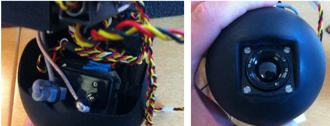
Figure B.10: Camera with sturdier mounting screws, USB and coax connectors.
