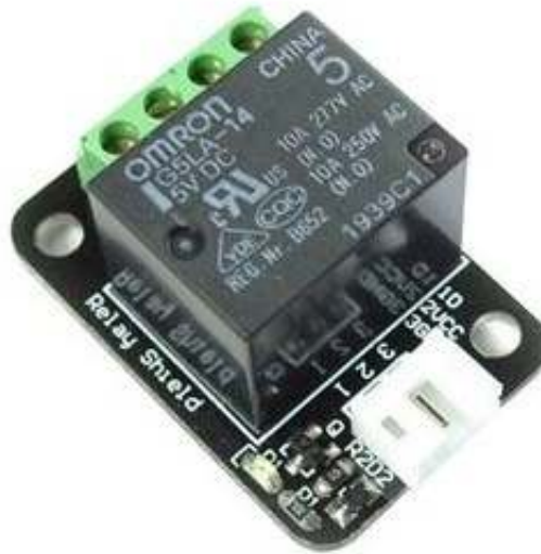
Figure C.9: DFRobot relay circuit used in the payload's cut-off circuit.
