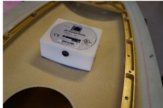
(b) The camera installed in the fuselage.
