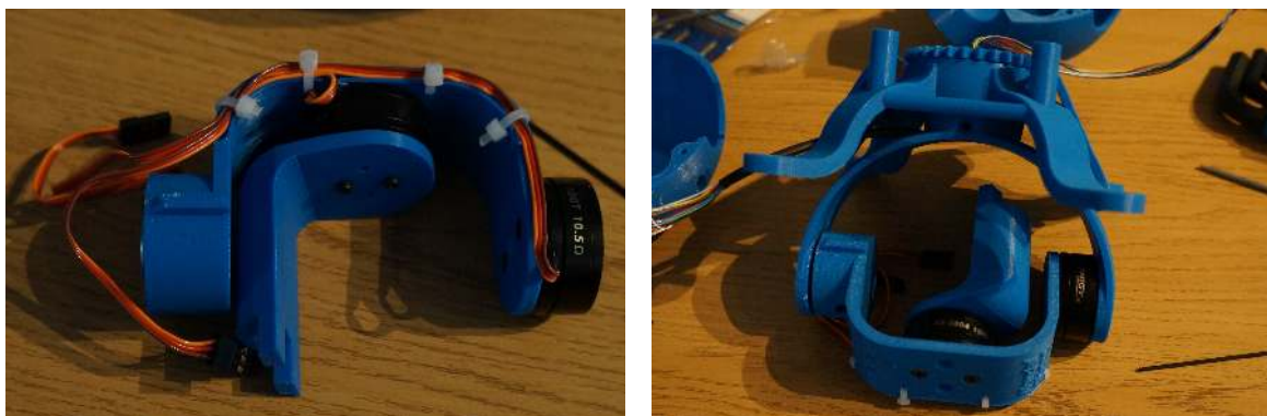
Figure B.22: Installing the roll arm and joining the upper and lower assemblies.
