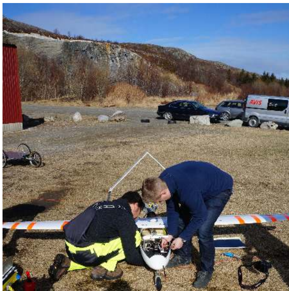
(c) Payload being installed in the UAV.
