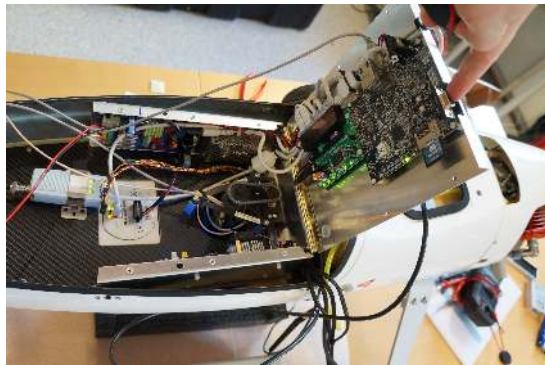
(a) Payload housing mounted in the UAV, housing lid opened.
