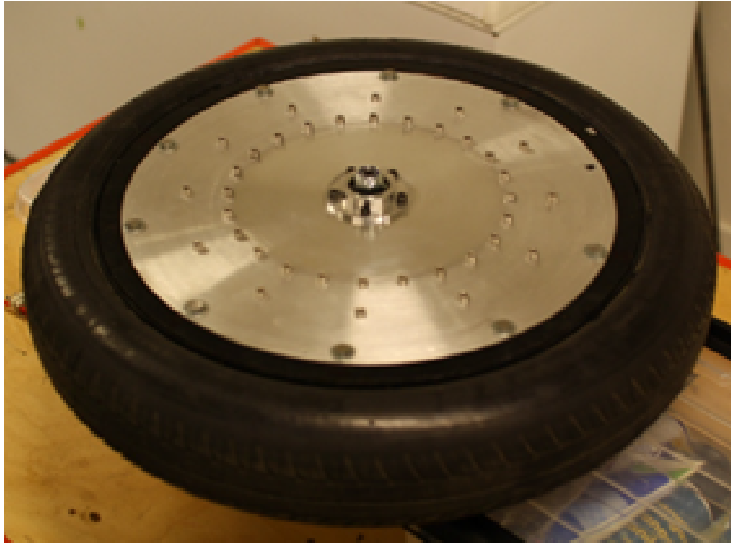
Figure 12: The in-wheel motor for the UrbanConcept, photo by Eirik Heien Mo.
