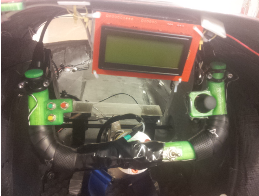
Figure 15: The steering wheel in the Prototype car. Buttons at the upper left, joystick at the upper right.
