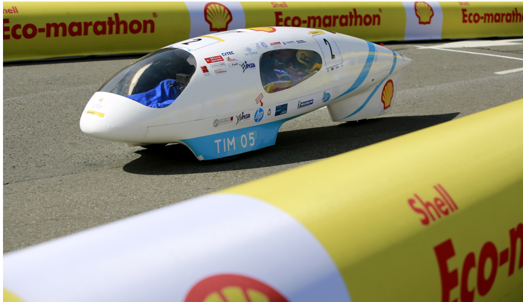
Figure 2: Example of the most common shape for prototype cars, the TIMO5 from Toulouse, France. All Rights Reserved Shell Eco-marathon 2014.
