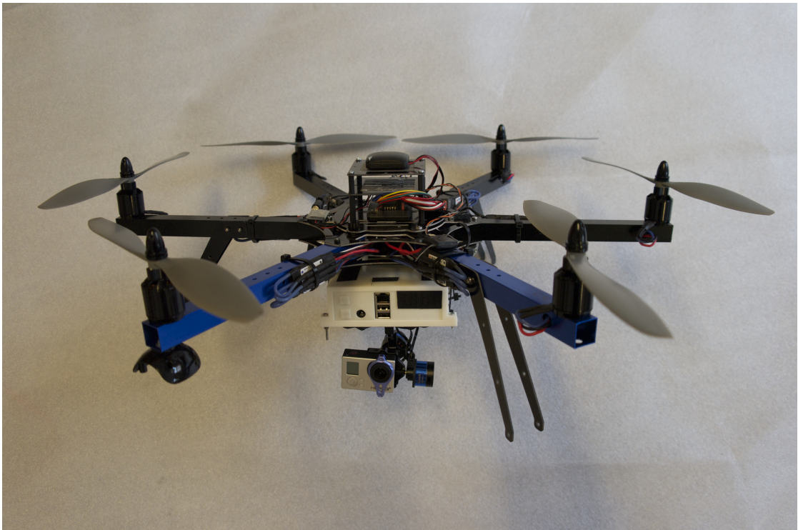
Figure 3.9: Photograph of the hexacopter. Here, the gimbal is used to stabilize the GoPro Hero3, as the infrared camera is not used. The Pandaboard is located within the white box hanging under the hexacopter. Photo by Thor Audun Steen
