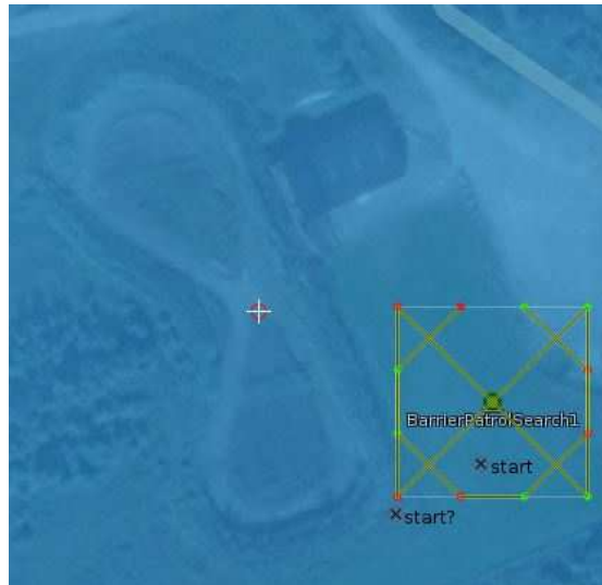
Figure 9.15: The barrier patrol search pattern tested at Agdenes.
