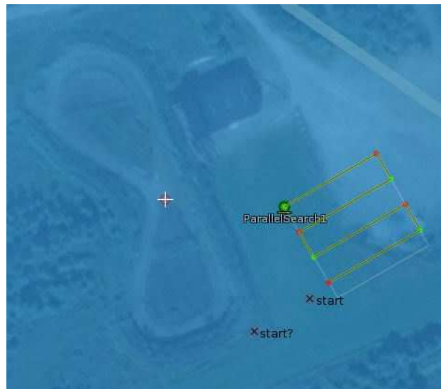
Figure 9.3: The parallel search pattern tested at Agdenes.
