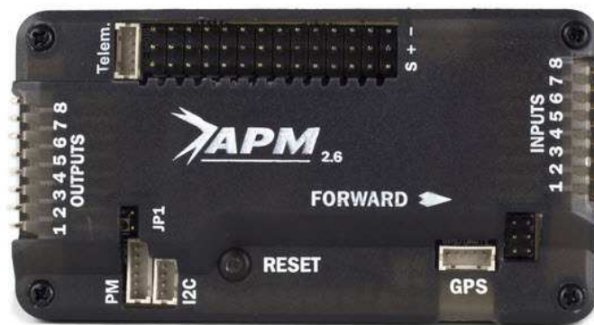
Figure 3.3: ArduPilot Mega 2.6. Image courtesy 3drobotics.com
