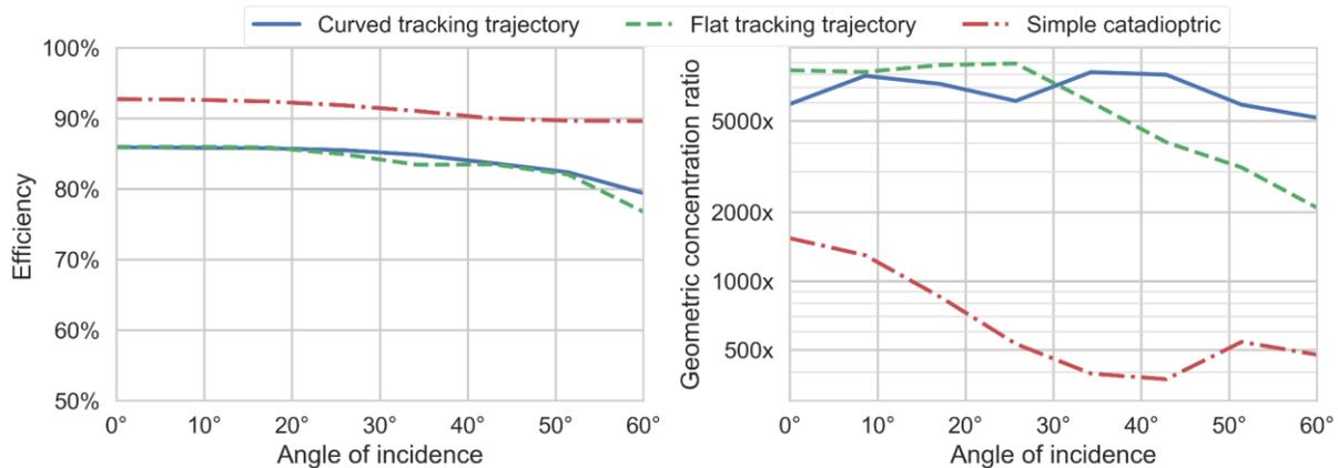
**FIGURE 5.** Simulated optical efficiency and geometric concentration ratio across tracking range for the optimized CPV configurations. The performance is simulated using Monte Carlo ray-tracking, taking into account reflection losses, chromatic aberration in the PMMA lens arrays, and the angular divergence of sunlight. The material is assumed to be non-absorptive.
