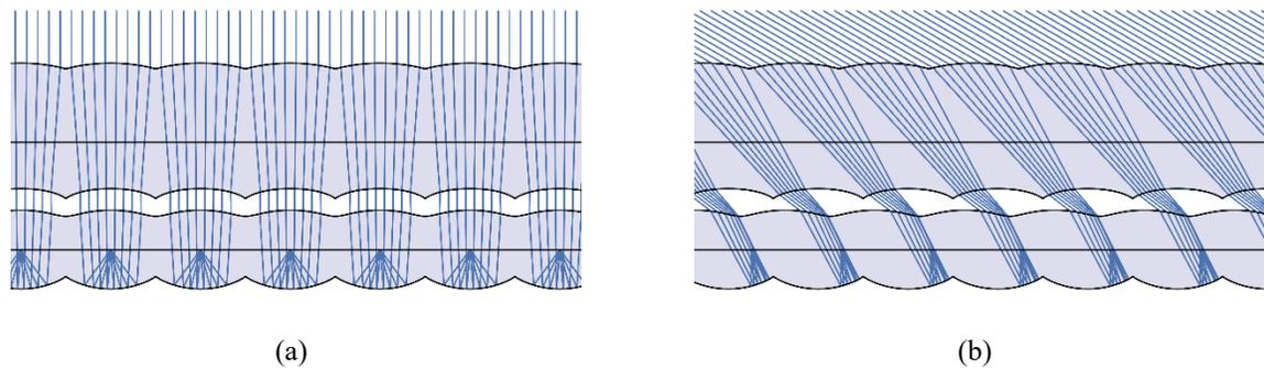
**FIGURE 3.** Optimized CPV-system with flat tracking trajectory at  $0^\circ$  (a), and  $60^\circ$  (b) angle of incidence.
