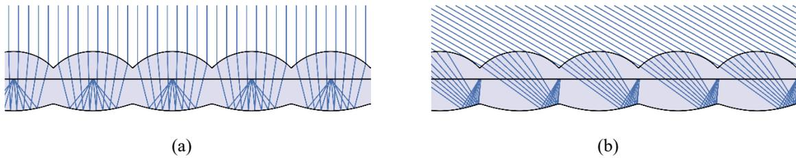
**FIGURE 2.** Optimized simple catadioptric CPV-system at  $0^\circ$  (a), and  $60^\circ$  (b) angle of incidence.
