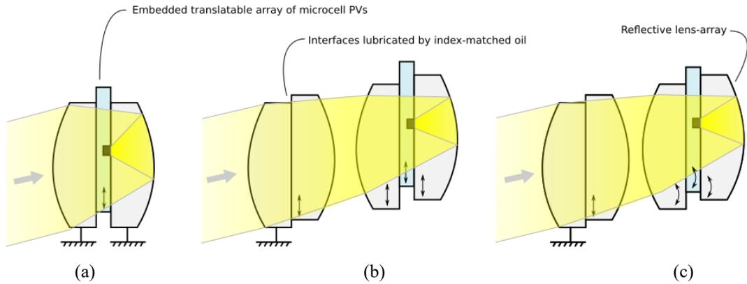
**FIGURE 1.** Conceptual illustration of the three different CPV-configurations that were optimized: Simple catadioptric (a), flat tracking trajectory (b), and curved tracking trajectory (c). In each configuration, the lens stacks are assumed to be arranged in a hexagonally packed lens array.
