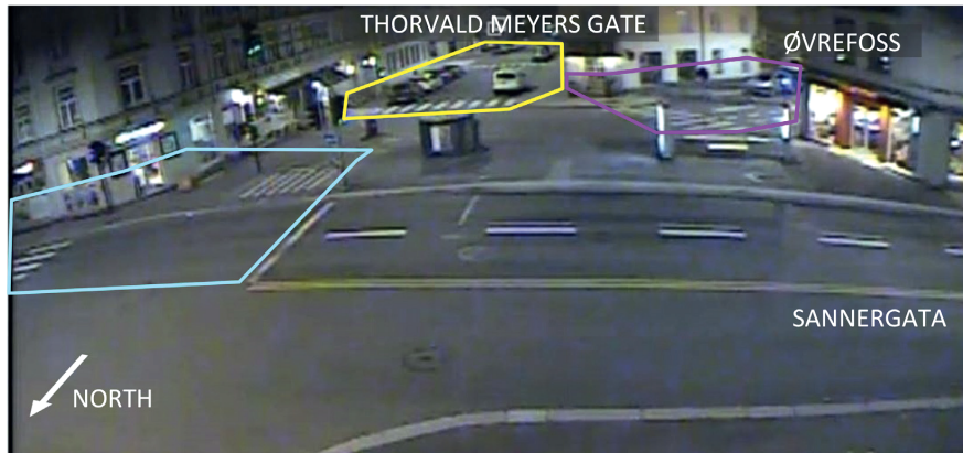
Fig. 4. Video camera perspective with bicycle counting zones for automated counting of bicycle movements between the three zones.
