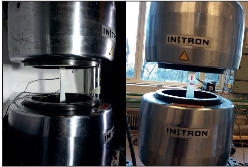
Figure 2.13. Placement and failure of the specimen in the test machine.
