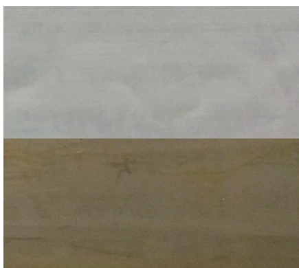
Figure 2. Visual inspection of an epoxy resin showing discoloration due to hygrothermal aging. Top: initial (blueish grey); bottom: redried after conditioning (yellow).
