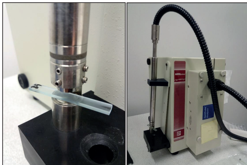
Figure 2.9. Epoxy sample analyzed with transmission FT-NIR spectroscopy (left) and FT-NIR spectrometer (right).
