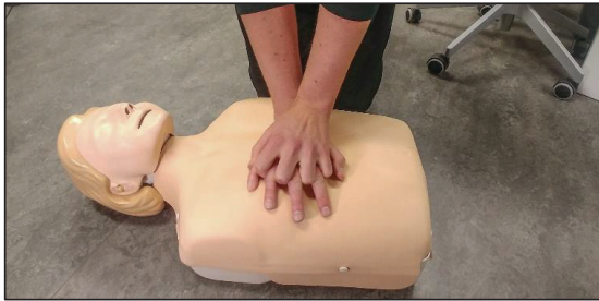
Fig. 2. Example of one commercially available resuscitation mannequin. This uses a linear compression spring mechanism to enable chest compressions.
