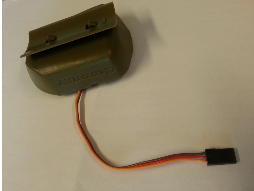
Figure 7.2: Quantum RTR Bomb System 1/6 scale plug-n-Drop. The brown cable is for ground, the red is for V_{CC} and the orange is for the signal
