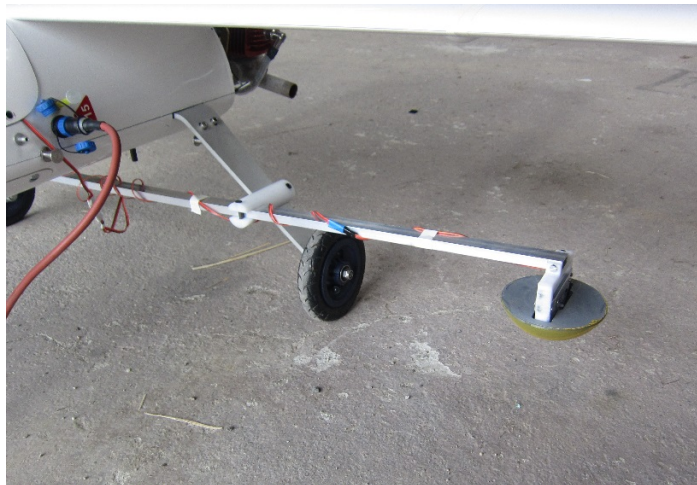
Figure 7.13: The metal bar with the drop mechanisms on it is attached to the UAV wheel assembly bars with two plastic joints.
