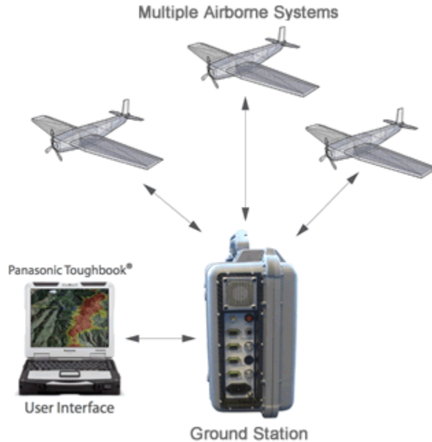
Figure 3.4: The Piccolo ground station communicates with the autopilots onboard the unmanned vehicles using radios, and with the user interface either wired or wireless. (source: Cloud Cap Technology (2014a) ).
