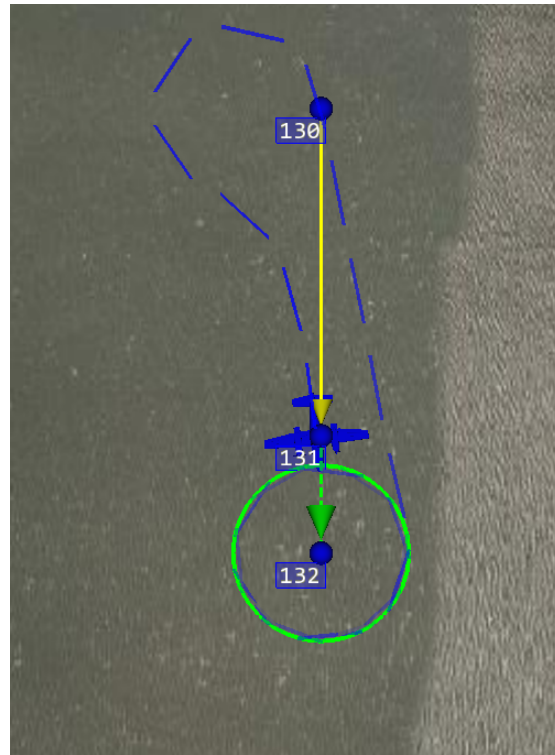
Figure 10.6: HIL simulation of the Straight Line Approach.
