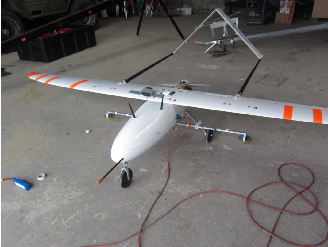
Figure 10.8: The Penguin B with the drop mechanisms mounted under its wings and the antennas on top of the fuselage
