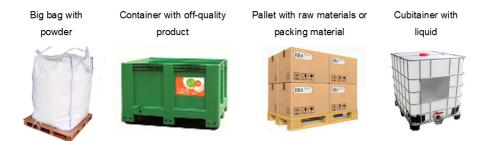
Figure 2. The most frequent loads transported with pallet movers.
