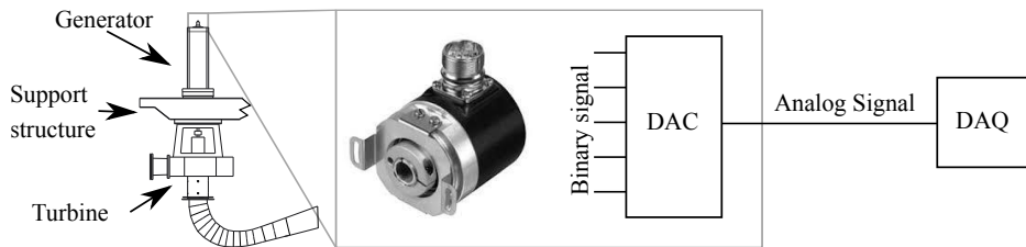
Figure 31 Position sensor on the shaft
