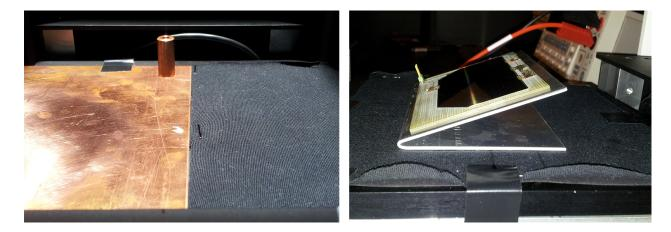
Figure 6.27: Photos showing the replacement work plane surface with lower reflectivity.
