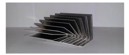
Figure 6.23: Photo of the mounting angles used for measuring at non-normal angles inside the solar simulator.
