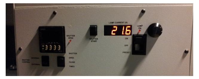
Figure 6.3: Photo of solar simulator control panel
