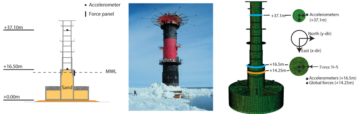
Figure 2. Illustration, picture and finite element model of the Norströmsgrund lighthouse, from Nord et al. (26).
