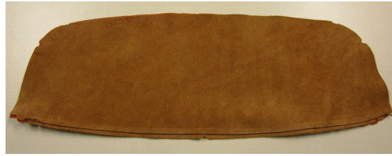
Fig. 12. The assembly of two parts as sewn in the experiment with two robots. The seam runs from left to right and is nicely placed at a nearly fixed distance from the edge. At the end of the seam an accumulated error of the feeding can be observed as a longitudinal displacement between the corners of approximately 10 mm.
