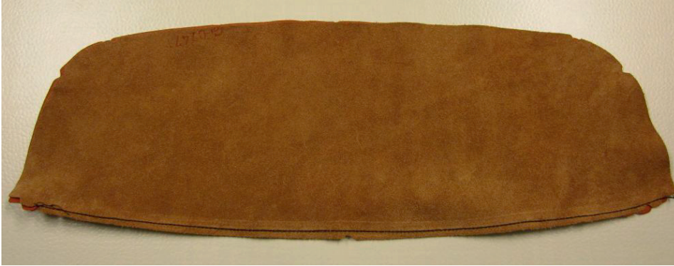
Figure 5.21: The assembly of two parts, sewn in the experiment with two robots. The seam runs from left to right and is nicely placed at a nearly fixed distance from the edge. At the end of the seam an accumulated error of the feeding can be observed as a longitudinal displacement between the corners of approximately 10 mm.
