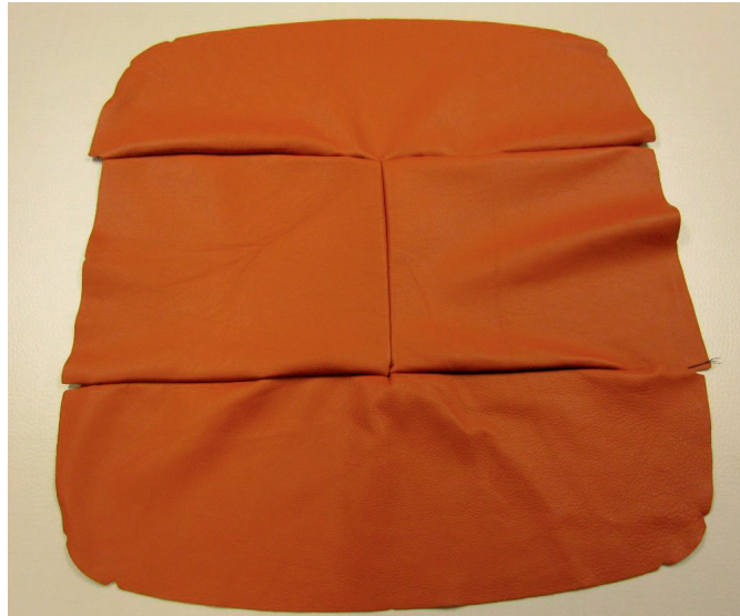
Figure 5.23: An assembly of four parts that have been sewn in the sewing cell. The handling before and after the sewing operation has been done manually while the sewing operation was fully automated.
