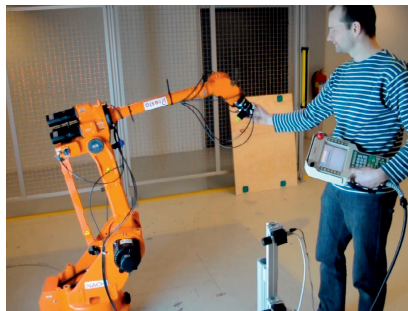
Fig. 3 Force control: The robot can be controlled by moving the tool.
